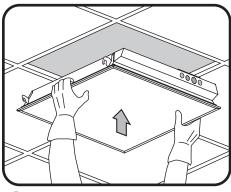
Install the fixture back to the ceiling. Connect the AC and dimming wires.
