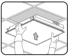
Install the fixture back to the ceiling.
