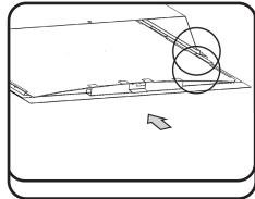
Slide in the new door frame. Ensure the outward frame bends are secured to the fixture housing. For door frames with sensors, partially install the new door frame. Connect the sensor wiring, then complete the door frame installation.
