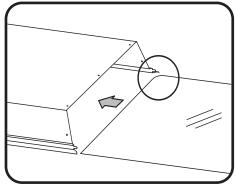
Slide in the new diffuser. Make sure the round corner on the diffuser slides in first as shown in the circled area of the above picture.
