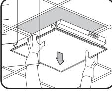
Disconnect the AC and dimming wires. Remove the fixture from the ceiling fixture.
