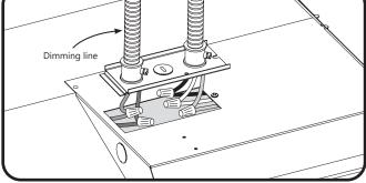
Install listed electrical fittings in the knockout holes for wire protection. Connect the dimming control (grey and purple or purple and purple/white) wires of the LED driver using 18-14AWG twist-on wire connectors.
