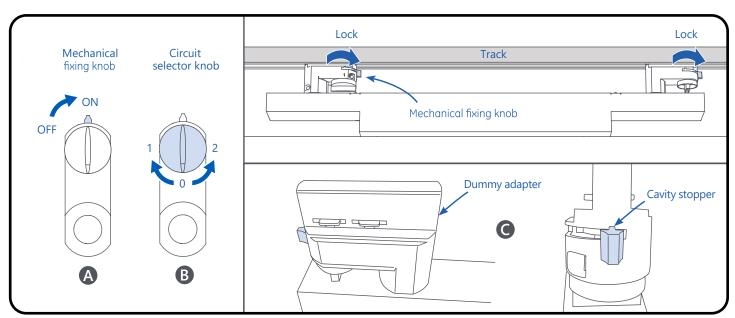
(A) On both adapters, rotate mechanical fixing knob clockwise to ON position to lock fixture to track.
