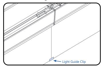
Push the inter-connector into the luminaires.
