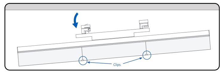
To remove fixture put Circuit Selector to 0 and Mechanical Knob to off. Then, while tilting fixture, remove luminaire marked side first. Carefully check the clips are still in the right positions after removing the protective film. If the clips fall down, need push them back to the right positions.
