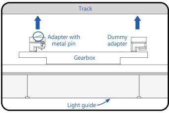
Ensure alignment lines on luminaire and adaptors are parallel and insert fixture vertically into track.
