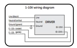
Risk of damage: Make sure that dimming cables are connected to proper driver inputs. Wrong connection may cause damage to the product.
