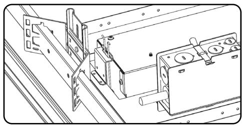
Carefully tuck the electrical conduit into the ceiling. Compress the torsion springs on the side of the fixture and insert them into the brackets on the rough in kit. Ensure that springs are properly inserted into the mounting brackets. Push the fixture up until it is flush with the ceiling.
