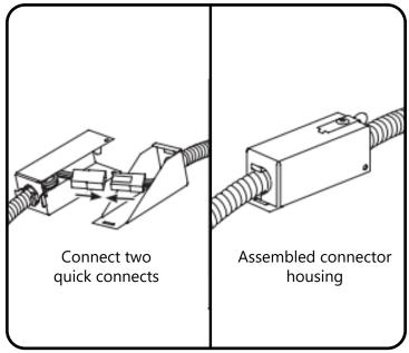
Connect the quick connect from the Rough in Kit to the quick connect on the luminaire. Assemble connector housing.
