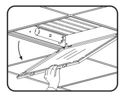
Swing down panel and lift off front bezel.
