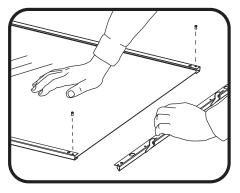
Place front bezel with diffuser on table. Unfasten the two rail screws on the end rail with latches, then remove this end rail.
