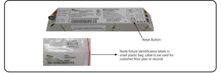
**LABELS:** The labels are in a small plastic bag and can be visible either on the control unit itself or near the fixture labels on the outside of the luminaire. These labels can be left in the same visible spot, or they may be placed in an area that is more convenient for identification.
