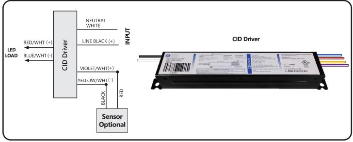
**NOTE:** CID Driver has "DALI Style" Lead (Yellow/White and Violet/White). These are NOT to be used for 0–10V dimming.
