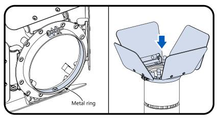
Slide the barn door accessory over the top of the fixture, ensuring that the flexible silver metal ring on the inside of the accessory sits completely around the outside of the fixture.
