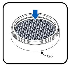
Place the hexcel louver inside the cap so that it rests on the inner lip of the cap.
