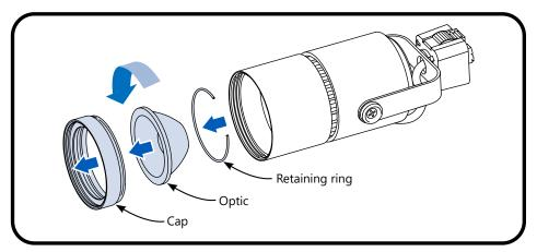
Unscrew the top of the fixture and remove the optic and retaining ring.
