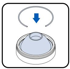
Replace the optic and retaining ring inside the cap.
