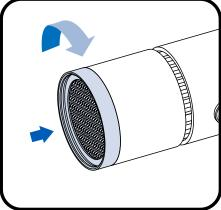
Screw the cap back onto the fixture.
