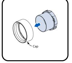
4 Place the accessory ring back inside the cap, snoot first.
