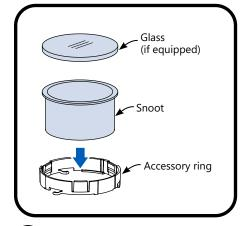
Gently push the snoot inside the accessory ring until it snaps into place, so that it sits evenly inside the ring. If the LTM fixture is equipped with Whiter White, the glass lens should sit on top of the snoot.
