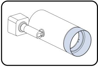
The snoot is secure when it is fully seated in the fixture.
