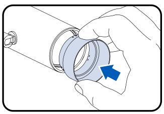
Gently slide the snoot into the front of the fixture with the smaller diameter down.
