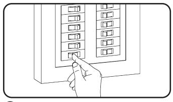
PRIOR TO INSTALLATION: Turn off power to fixture.
