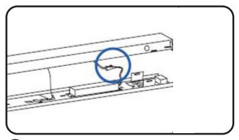
CONNECT DRIVER TO MAIN FEED NOTE: For sensor SKUs, Please ensure the sensor is properly secured prior to installing the LED panel. CAUTION: For sensor SKUs, Please be careful with handling. Keep hand far from sensor location while installing.
