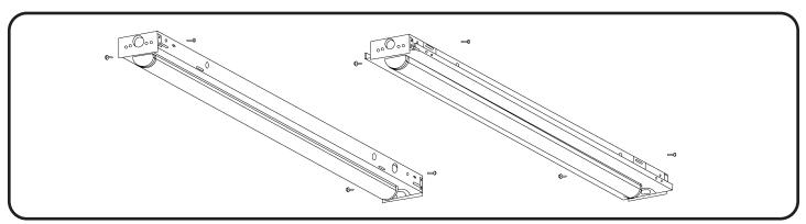
SECURE LED PANEL TO FIXTURE HOUSING: Once driver is properly energized, adjust bracket by opening or closing to snugly fit against fixture housing and secure LED panel to fixture housing by using the provided #8x1/2" self drilling screws. If there are no brackets, then use the #8x1/2" self drilling screws to secure the LED panel directly to the fixture housing.
