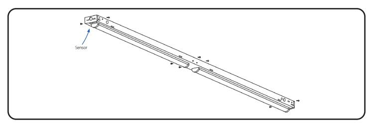
SECURE LED PANEL TO FIXTURE HOUSING (8ft. Kits): Connect the driver LED panel to the support LED panel using the 2 halves of the connector. Once driver is properly energized, adjust bracket by opening or closing to snugly fit against fixture housing and secure LED panels to fixture housing by using the provided #8x1/2" self drilling screws. If there are no brackets, then use the #8x1/2" self drilling screws to secure the LED panels directly to the fixture housing.
