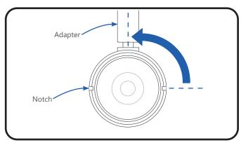
Remove old lens: Rotate the cap 90 degrees counter-clockwise until the notches fully align with the adapter and pull out.
