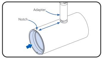
Install the new lens: Align notch with the adapter.
