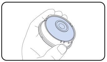
Inspect field changeable lens to ensure no dust particles are trapped inside.
