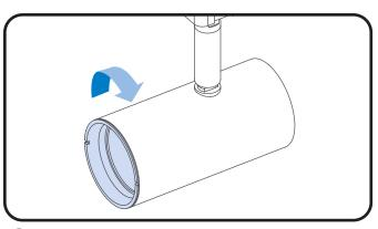
(5) Rotate lens 90 degrees clockwise to lock it in place.
