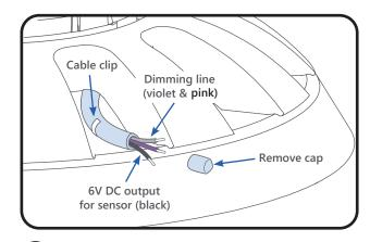
If dimming wire connection is required, pull out the dimming wire from cable clip, and carefully press back plastic cover on the heatsink. **NOTE:** Must strip the cable jacket. Also need to strip off 10mm from the violet and pink wires. **NOTE:** Must use waterproof connector to connect the dimming wire.
