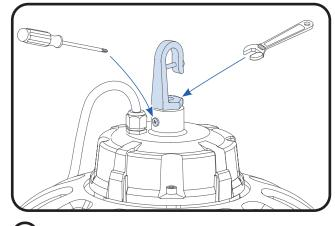
First, unfasten the M4 screw of luminaire and carefully tighten hook on the luminaire by tool. Fix anti-rotation M4 screw to secure the hook to the fixture.
