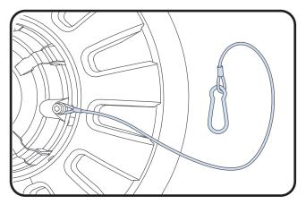
4 Optional: To install safety tether, unfasten one screw from driver enclosure and put the safety tether on the bolt. Use screwdriver to secure tether to the driver enclosure and heatsink.
