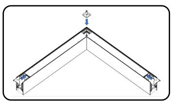
Place bracket with cable gripper in corner. Slide remaining brackets down fixture.
