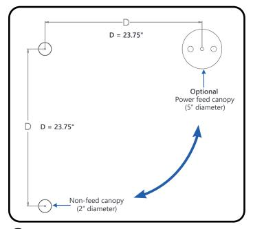
For T-Grid installation, use hardware provided with fixture and starter kit. For drywall installation, 1/4"-20 threaded rod should be provided and installed by other.
