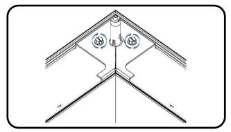
Secure brackets together with the two screws provided.
