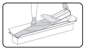
Carefully unpack unit from its packaging. Properly inspect for defects before installing. Wear work gloves to prevent dirt and oil from being transferred to the luminaire.
