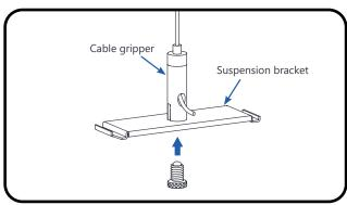
Connect cable gripper to suspension bracket using provided screw. Feed cable into top of cable gripper and pull through.
