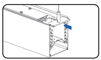
Slide second suspension bracket into opposite side of fixture and level fixture.
