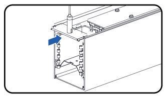
Slide suspension bracket into housing.
