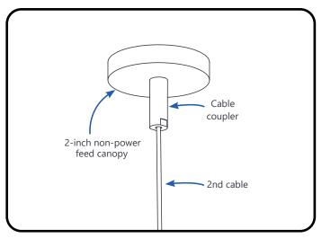
Hang cable from a structural ceiling member capable of supporting the weight of the fixture and cover with canopy.
