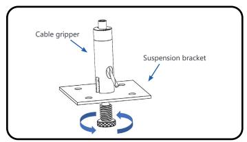
Connect cable gripper to suspension bracket using provided screw. Feed cable into top of cable gripper and pull through.
