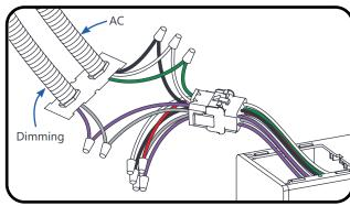
Connect to the AC line from fixture with twist-on wire connectors to conduit line. Repeat for dimming line. Cap unused wires. See *Wiring Section* for details.
