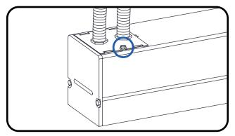
Reattach knockout plate with conduit attached to fixture with screws.
