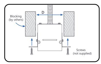
Screw luminaire to existing blocking.
