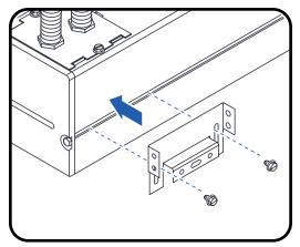
Check bracket height and install the screws in the same hole location. Install four mounting brackets (one per side) into grooves on both sides of luminaire. Position bracket within 1/8-inch from ends.
