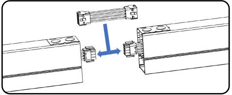
For continuous installations where the harnesses do not mate; use the supplied jumper harness to connect fixtures.
