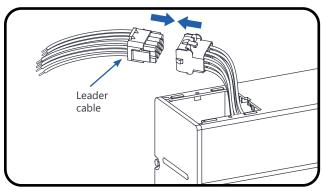
Connect leader cable to the AC line by clipping harness connectors together. Repeat for dimming leader cable.
