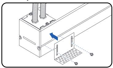
Attach 4 drywall brackets to luminaire (one per side) with provided screws. Bracket installation height is flexible to accommodate various drywall thicknesses and fixture installation depths.
