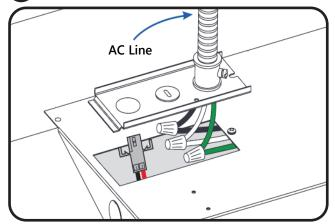
Connect sensor cable to luminaire or accessory box. If the sensor cable is not mounted on the knockout plate, remove the knockout plate to access the sensor cable. The luminaire or accessory box will have a black and red cable with a male connector located inside the electrical cavity. Remove a knockout hole on the knockout plate. Follow appropriate codes for type of grommet to be used for the sensor cable to pass through the hole.
