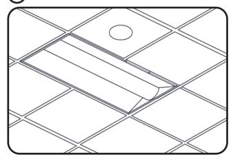
Make hole in ceiling to accommodate a standard UL listed electrical enclosure compatible with cover plate.
