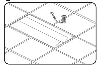
Depending on sensor mounting, route cable through created hole in ceiling. Make sure sensor is connected to the cable.
