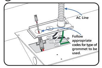
Route the sensor cable through the knockout hole and/or bushing into luminaire and make the connection. Fasten the knockout plate back to luminaire. All work happens above ceiling. The luminaire does not have to be removed.
