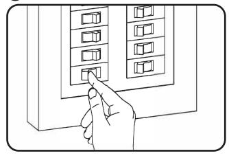
Remove power by switching circuit breaker to the off position.
