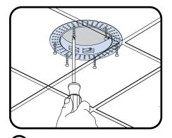
Ensure that muddy frame is lined up with rig frame and secure it to the ceiling using fine thread  $6 \times 11/4 \#2$  drywall screws (not included). Prior to plastering and painting, insert the light reflector to ensure that reflector is fush with the ceiling. Repeat step 4 for height adjustment if needed.
