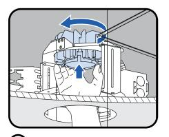
Remove LED module by pushing up, then counterclockwise to disengage 3 clips.
