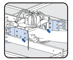
Adjust fixture height to be flush with ceiling and secure by tightening both adjustable mounting bracket wingnuts.
