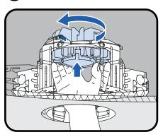
Remove LED module by and pushing upward and then counterclockwise to disengage 3 clips.
