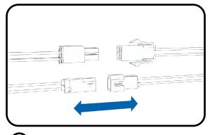
8 Disconnect AC connections, dimming and test button.
