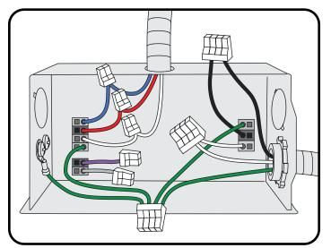
**Optional:** If using a 0-10V dimming controller, connect matching-colored wires together.
