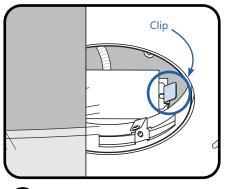
3 Disengage driver by pulling on clip.
