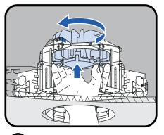
3 Reach inside and push LED module upward and then counterclockwise to disengage 3 clips.
