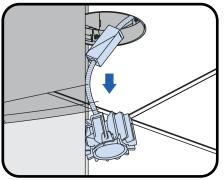
3 Remove LED module from frame, bringing below the ceiling plane.
