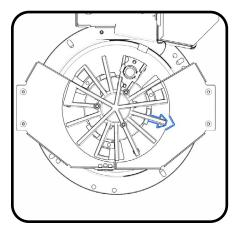
Note: Align both arrows before installing the light engine. Once both arrows are aligned, push the LED module and then rotate it clockwise to engage 3 clips.
