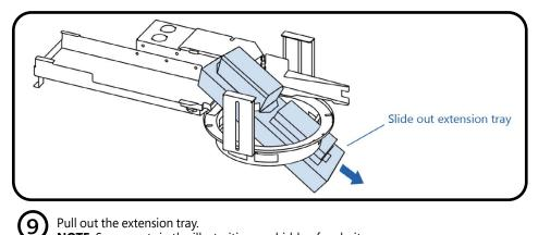
Pull out the extension tray. NOTE: Some parts in the illustraition are hidden for clarity.
