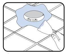
D Plaster onto the muddy frame and ceiling. Repeat plastering process if needed. Sand and paint once plaster is set.
