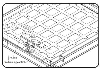
Connect the AC line to the black (line) and white (neutral) input wires of the LED driver using 18-14 AWG twist-on wire connectors. Connect the ground wire to the green-yellow ground wire of the LED driver. When connecting dimming controller, wires must run through a separate knockout hole equipped with an appropriate wire restraint or cable gland. Then, re-attach and fix enclosure cover with screw by screw driver.
