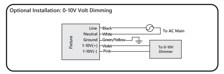
Option for Step 2: Follow diagram for 0-10V. Run wires from controller through a different knockout than the AC input wire. At output side of fixture, make appropriate connections using twist-on wire connectors. To combine with LFAMBAOVQFAEL, LCAMBAONRFAEL, LCAMBAOTSFAEL, LCAMBAOTQFAEL, LFAMBADVQFA, LCAMBAONRFAB2, LCAMBAOTSFAB2, LCAMBAOTGFAB2, LCAMB
