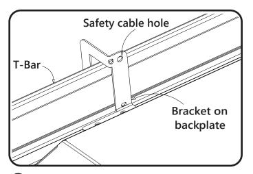
Bend the brackets on the back plate to make sure they hook to T-Bar.
