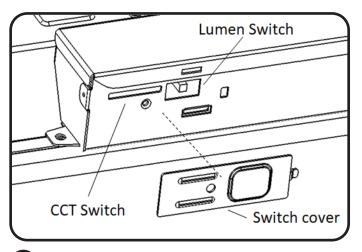
Remove the fixture from the package. Default lumen level is H(high), default CCT is 4000K. If a lumen level other than H(high) is desired, or CCT other than 4000K is preferred, remove switch cover and set to the desired lumen level, or preferred CCT by screwdriver, then re-attach cover.
