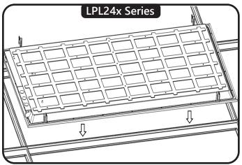
Insert luminaire into T-bar ceiling grid. Unit should not move freely within the ceiling grid. To ensure a consistent appearance, align fixtures in the same orientation throughout the ceiling pattern.
