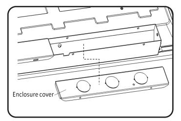
Remove electrical enclosure cover. Carefully remove knockout for AC line input wires. Install listed electrical fittings in the knockout holes for wire protection.
