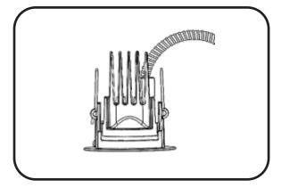
Deflect the springs on the luminaire into an upright position.
