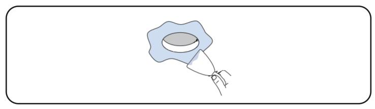
Plaster Mud Frame. Ensure Reflector is flush with plaster . Sand and paint once plaster is set.
