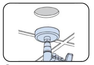
Cut the appropriate size hole into ceiling. Refer to Hole Requirements section.
