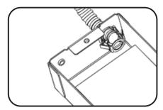
CAREFULLY REMOVE LIGHT ENGINE from ceiling and pull Driver Enclosure below ceiling. Un-screw driver enclosure cover, disconnect DC wires from driver. Compress Tabs on DC Conduit holder and remove conduit from Driver Box.
