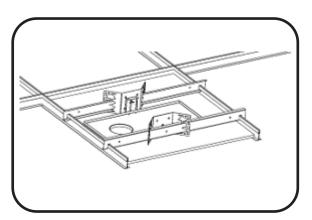
Mount Hanger Bars onto T-Grid.
