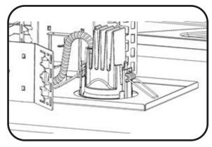
Push the fixture through the hole in the ceiling. Ensure that the springs are engaged on the frame and it is held securely.
