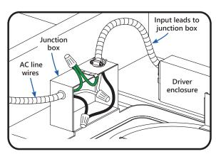
Connect AC conduit to driver enclosure. Ensure that connections are secure. Conduit connected to the driver enclosure must still allow for the enclosure to be removable from the ceiling. Connect the black, white, and green AC line wires to the appropriate wires inside driver enclosure. Connect optional dimming wires as needed. Securely close driver enclosure. Connect AC conduit to pre-existing electrical enclosure and securely close.
