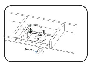
2 Remove existing lamp, reflector and conduit.
