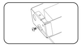
Detach the safety tether connecting the light engine to the driver box. Connect conduit and safety tether that come with new light engine to driver box. Reconnect DC Wires to driver. Ensure that all mechanical and electrical connections are secure. Close driver box using exiting screw and re-install luminaire.
