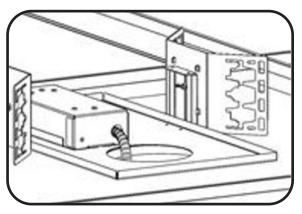
Position the driver enclosure into the ceiling through the existing opening. For new construction installation, ensure driver is on rough in kit (see page 4 for more information).
