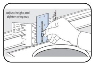
Adjust height and tighten the wing nut. Ensure rough in plate is flush with ceiling. To Continue Installation, go to the Luminaire Installation section, Step 3.
