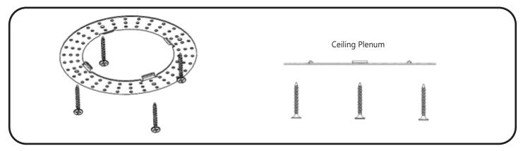
Ensure that Mud Frame is lined up and centered in ceiling hole. Secure to ceiling using fine thread 4 x1 ¼ #2 drywall screws (not included). Ensure that the holding tabs are above the ceiling surface.
