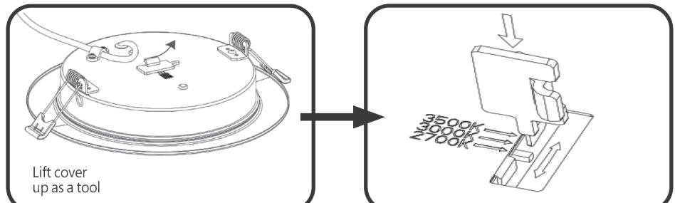
**NOTE:** For 2700/3000/3500K model and 3500/4000/5000K model , the default CCTs is 3000K and 3500K respectively. Lift up the cover for the switch, and use it as a tool to choose the desired CCT.
