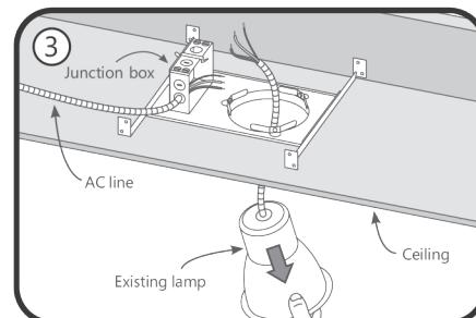
Remove existing lamps, fixture and ballast. Disassemble AC conduit from the existing junction box. Verify that the AC supply line is provided with a ground wire connected to the luminaire.
