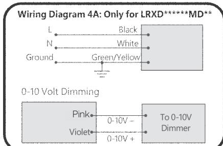
Optional dimmer: When connecting with dimming controller, wires must be run through another separate knockout hole. Connect the violet (dimming +) and pink (dimming -) wires to the violet and pink wires of the fixture.
