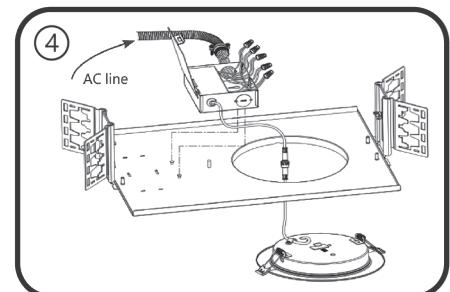
Secure provided junction box to the building structure or existing frame per local codes. If necessary, remove existing junction box. Connect AC conduit to provided junction box and connect the black, white, and green/yellow wires of the AC leads to the black, white, and green wires using twist-on wire connectors and close junction box.
