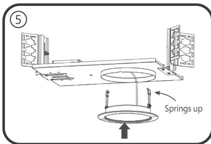
Load springs into upright position by twisting the springs upward and carefully insert the fixture to the hole of the frame. Verify the trim is flush with ceiling.
