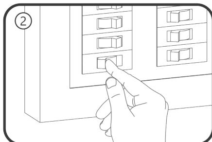
Ensure that the power to the unit is turned off. Use proper lockout and tagout procedures.
