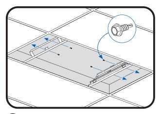
Install PVR Mounting Bracket to each end of the fixture by sliding PVR Mounting Brackets between the fixture and T-grid, ensuring the mounting bracket is centered in the fixture. Secure the PVR Mounting Brackets to the fixture using 4 of the provided #8x1/2" self-drilling screws.
