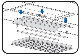
Prior to installation, disconnect all incoming power to fixture. Remove existing hardware (lens/lens frame, parabolic louver, reflectors/ballast covers, brackets, lamps/ lamp holders). Leave supply and grounding leads.
