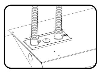
Replace electrical enclosure cover and secure it with the screw.
