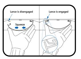
The diffuser panel may become loose during shipping or if the PVT luminaire is significantly twisted during installation. It is important to ensure the diffuser is completely engaged to avoid it falling out after installation is complete. If diffuser is loose, grasp the diffuser and gently squeeze together the re-engage over lances.
