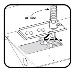
Install listed electrical fittings in the knockout holes for wire protection. Connect the AC line to the luminaire internal wires according to the wiring diagrams using 18-14AWG twist-on wire connectors.
