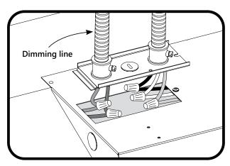
Install listed electrical fittings in the knockout holes for wire protection. Connect the dimming control (pink and purple or purple and purple/white) wires of the LED driver using 18-14AWG twist-on wire connectors.
