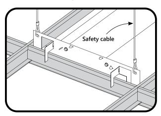
Bend the 4 clips to secure the luminaire in place. Install the safety cables through the holes on the clips (per local building codes, safety cables supplied by others).
