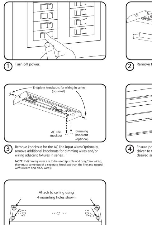
Use the four existing holes in the housing to drill four fasteners (optimal for the type of ceiling present) directly into the ceiling, one fastener in each hole. Each fastener should be rated to hold at least 11 pounds.
