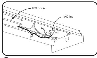
Connect the AC line to the black (line) and white (neutral) input wires of the LED driver using 18-14WG twist-on wire connectors. Connect the green (ground) wire to the ground screw of the housing.
