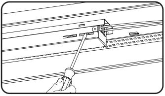
Ensure power to the fixture is turned off. Use a screw driver to toggle the Lumen and CCT switches to the desired settings.
