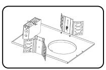
G Mounting brackets could also be fixed on the short side of frame.
