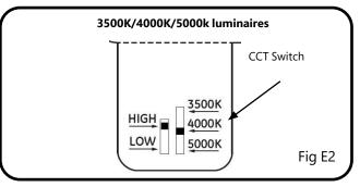
**NOTE:** For 10in and 12in fixtures, the CCT switch is located on the housing sealed by a plug, and the cover of the lumen switch can be used as a tool to select lumen and CCT. See fig E4.
