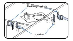
Place side L-brackets on existing В frame screws and tighten with screwdriver on both sides of the frame. Then attach mounting brackets to both L-brackets with wing nuts (provided).
