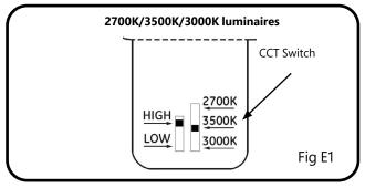
**NOTE:** The cover of the lumen/CCT switches can be used as a tool to select lumen and CCT. See fig E3.Place the switch cover back after lumen and CCT setting.
