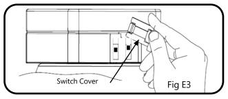
**ONLY FOR 10IN AND 12IN FIXTURES:** The CCT switch plug must be placed back after CCT selection to avoid light leakage and dust/bug ingress. See fig E5.
