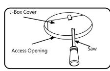
Cut an appropriate hole on the A ceiling tile according to Tab 4. Ensure the ceiling hole diameter match the frame opening diameter.
