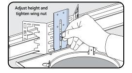
Adjust fixture height to be flush with Æ ceiling and tighten both mounting bracket wing nuts.
