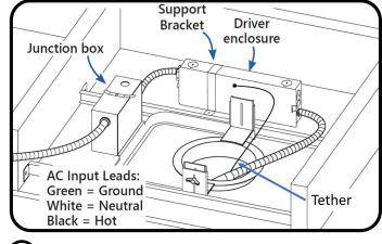
Place the driver enclosure portion of the fixture assembly in the ceiling next to the rough-in kit so that the input leads are in close proximity to the driver enclosure.
