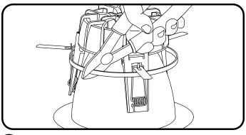
Cut cable tie on fixture so that the fixture is ready to be installed.
