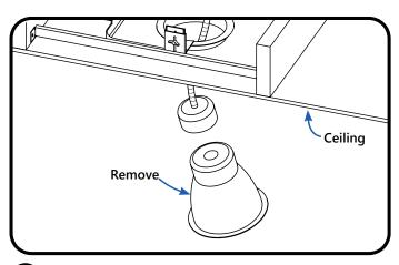
Remove existing lamp and reflector.
