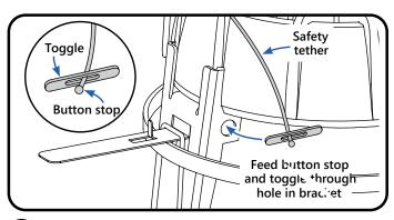
6 Attach the other end of the safety tether to the fixture using one of the three holes located on the fixture brackets. Feed the button stop and toggle through the hole and slide into the hole in the bracket. Allow the fixture to hang freely.
