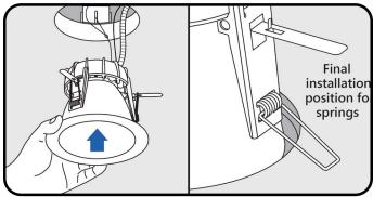
Push fixture through the hole in the ceiling. This will engage the protruding arms, thus, releasing the springs. The springs will draw the fixture up into the ceiling and hold it there tightly.
