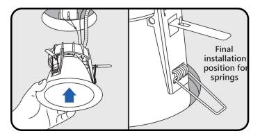
9 Push fixture through the hole in the ceiling. This will engage the protruding arms, thus, releasing the springs. The springs will draw the fixture up into the ceiling and hold it there tightly.
