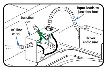
**NOTE:** Verify conduit to ensure no defect or openings on both the AC and DC conduits. Ensure DC conduit placement does not result in additional stress upon full installation of luminaire
