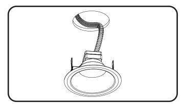
Insert LRXB Series fixture into ceiling.
