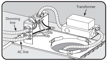
Connect the step transformer conduit to the existing AC and dimming leads in the junction box. Verify that the AC supply line and dimming leads are connected properly. If dimming leads will not be utilized, please do not remove the twist-on wire connectors.
