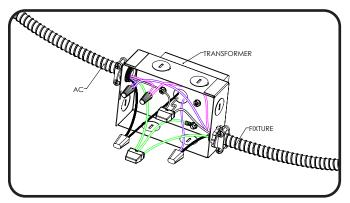
Carefully take out the 347V kit and fixture from different packages. Connect fixture conduit to the 347V kit J-box. Connect White wire (N) from fixture to White from kit. Black (L) from fixture to light purple wire from kit. Dimming wires connect to dimming wires from kit conduit.
