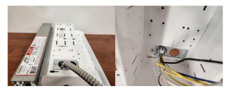
7) Place EMBB button bracket inside the housing next to the endcap and ensure button is visible from the exterior. Mount the button bracket using the screws provided on the interior side of the fixture as seen below, Screw position vary per body size, below are the 2 possibilities:
