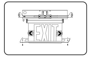
6 Insert fixture into metal box and snap by spring, fix trim plate on the metal box by 2 screws
