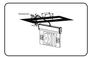
Make proper electrical connections at J-box in the metal housing, refer to "ELECTRICAL CONNECTIONS" You may need to use holding wire during wiring.
