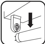
2 Remove all fluorescent lamps and ballast/wiring area cover. Cut the ballast lead wires about 6 inches away from each lamp holder.
