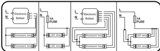
3-7 If two wires come from an existing lamp holder (rapid start type), these two wires should be wired or shunted together.
