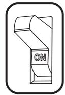
1) Ensure power is off to luminaire by disconnecting the supply voltage.
