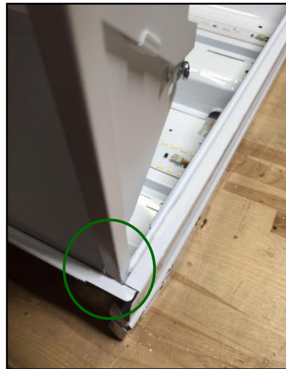
Figure 7. Hinges slid backwards towards side of housing.
