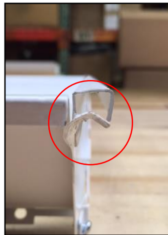
Figure 3. Hinge Front View (Incorrectly Aligned)
