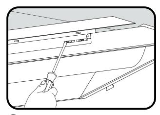
Ensure power to the fixture is turned off. Use a screw driver to toggle the Lumen and CCT switches to the desired settings.
