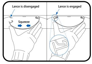
The diffuser panel may become loose during shipping or if the PVR luminaire is significantly twisted during installation. It is important to ensure the diffuser is completely engaged to avoid it falling out after installation is complete. If diffuser is loose, grasp the diffuser and gently squeeze together the re-engage over lances.
