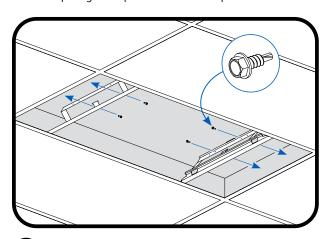
Install PVR Mounting Bracket to each end of the fixture by sliding PVR Mounting Brackets between the fixture and T-grid, ensuring the mounting bracket is centered in the fixture. Secure the PVR Mounting Brackets to the fixture using 4 of the provided #8x1/2" self-drilling screws.
