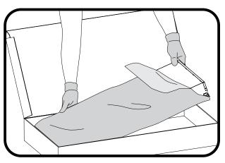
Carefully unpack unit from its packaging. Properly inspect for defects before installing. Wear work gloves to prevent dirt and oil from being transferred to the luminaire.
