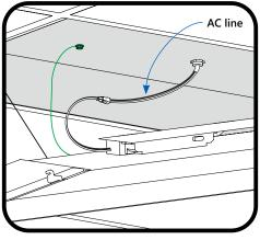
Connect the LED driver to AC line using the provided ballast disconnect. See "Electrical Connections" section for wiring details.
