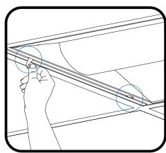
Secure swing door by locking latches found on the end of the assembled PVR Door.
