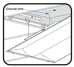
Install grounding wire using provided green ground screw (if existing hole is available) OR #8x1/2" self-drilling screw.
