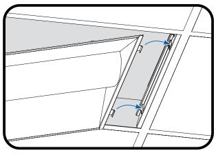
Install the PVR Fixture T-hinges into the PVR Mounting Bracket cutouts.
