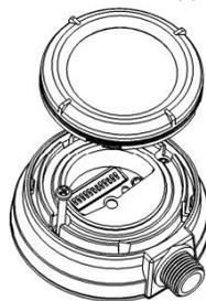
Fig. 1 – Lens Installation
