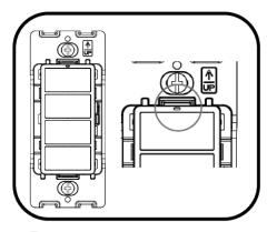
The device's LED flashing on for 2 seconds every 30 seconds indicates that the batteries need to be replaced.
