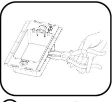
For proper installation into a dual gang junction box, the tabs between adjacent back housings must be removed. Carefully observe the correct orientation (the UP arrow should be in the upper right corner on each back housing). After double checking the product orientation, break off the necessary tabs using pliers.
