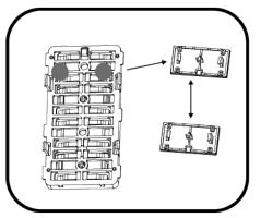
2 Press the replacement button module with the desired printing onto the device.
