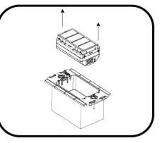
Remove the device from 2 the back housing.
