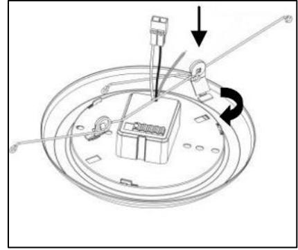
For installation into a 6in can, turn brackets outward, as shown
