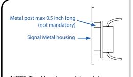
NOTE: The Hanging resistor plate is a Hot surface that must be kept away from plastic or wires. It is recommended to mount the resistor plate on the signal metal head using metal hardware. See suggested mounting picture above. Contact Current for more information.
