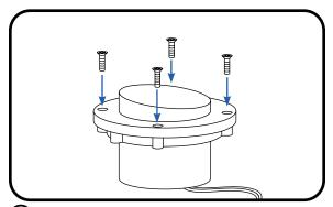
(4) Insert and fasten all four screws into the front shell. (Torque between 4 and 5 inch-pounds).
