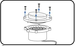
1 Lay down the lamp on a clean workbench on its back shell to ensure no scratches on the front shell. Remove the 4 top screws and pull the front shell off.
