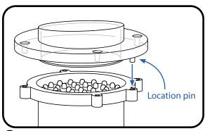
3 Using gloves, gently place the new front shell on the back shell. Align the lens location pin to the location pinhole on the back shell.
