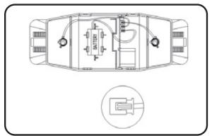
(3) Connect to the battery with connectors.
