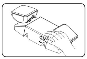
Install the housing to Base plate, turn on the AC power and press the "TEST" button check light.
