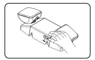
Align snaps and push housing directly onto the Base Plate. Apply continuous AC power and press "TEST" button to check light.
