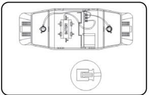
Connect the AC wires to the supply using the wire-nuts provided. Connect the battery.
