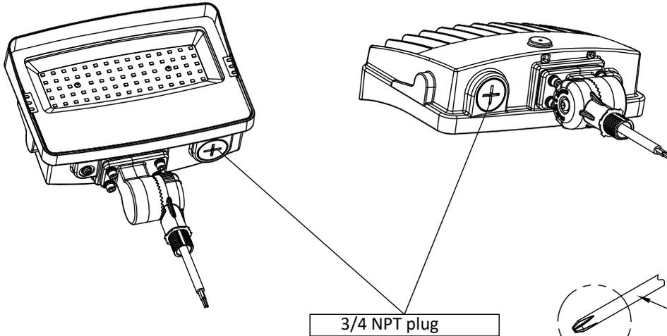
2. Remove plug with 6mm Philips screwdriver. Switch power and CCT as pictured on the left.
