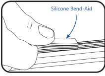
Fill the entire light guide channel with the GEXNBA Silicone Bend-Aid(s) and press into place. Bend-Aid must be installed prior to heating and forming. The GEXNBA Silicone Bend-Aid is reusable.
