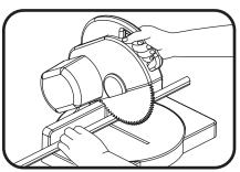
Cut the light guide to the required length using a hacksaw, chop saw (cross cut or veneer blade only), band saw, or other appropriate plastic cutting tool.
