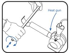
Part 1: Move the section back and forth while rotating about the diameter until it is soft and pliable. Gently bend to the desired angle. It is recommended to use a heat-deflecting shield to distribute the heat evenly. Avoid localized overheating that may result in distortion or damage (i.e. bubbling) of the light guide.
