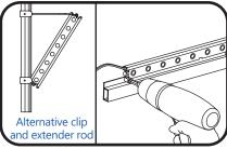
Arrange modules evenly spaced apart. Place the Tetra® modules on the Mounting Rail and secure into lip with a self-tapping #6 (M3) screw or 1/8-inch (3.175 mm) rivet. Or mount using the alternative clip and extender rod configuration.
