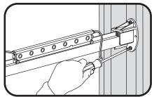
3 Secure the Mounting Rail to the inside of the box sign using a Tetra® Mounting Rail Clip or other suitable mounting means. Ensure the #6 (M3) screw does not exceed 3/4 inches (19 mm) in length.
