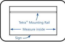
Measure and cut Tetra® Mounting Rail or other suitable mounting means to appropriate length to fit into sign.
