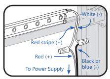
4 Connect the red stripe wire (+) of the LED system to the red wire (+) of the power supply. Connect the white wire (-) of the LED system to the black or blue wire (-) of the power supply.
