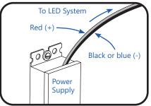
Run a wire from the power supply to inside the sign and connect to the first module on the strip.
