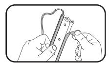
Peel off backing to expose adhesive tape.
