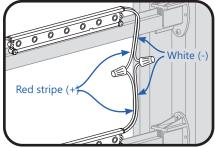
Connect modules using twist-on wire connectors or in-line (IDC) connectors. Join white wires together and red striped wires together.
