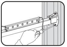
(3) Secure the Mounting Rail to the inside of the box sign using a Tetra® Mounting Rail Clip or other suitable mounting means. Ensure the #6 (M3) screw does not exceed 3/4 inches (19 mm) in length.
