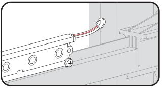
2 Cap all exposed wires with appropriate end caps or apply electric grade (non-corrosive) silicone for additional weather protection.
