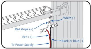
Connect the red stripe wire (+) of the LED system to the red wire (+) of the power supply. Connect the white wire (-) of the LED system to the black or blue wire (-) of the power supply.
