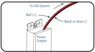
Run a wire from the power supply to inside the sign and connect to the first module on the strip.
