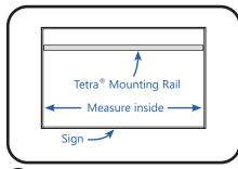
Measure and cut Tetra® Mounting Rail or other suitable mounting means to appropriate length to fit into sign.
