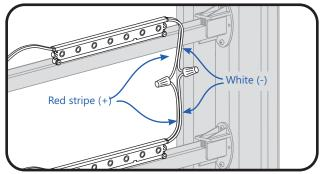
Onnect modules using twist-on wire connectors or in-line (IDC) connectors. Join white wires together and red striped wires together.
