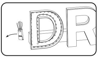
Remove the existing GECLPS3 or GECLPS4. Do not remove existing channel letters and wiring.
