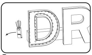
Remove the existing GECLPS3 or GECLPS4. Do not remove existing channel letters and wiring.
