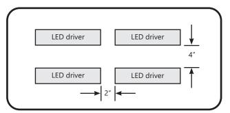
4 If installing multiple LED control modules or LED drivers in the same compartment, keep them at least 2" (50.8mm) apart end to end and 4" (101.6mm) apart along the sides.
