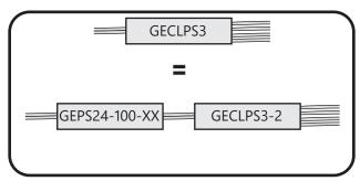
One GECLPS3-2 and one 24VDC, 100W, Class 2 Tetra LED Driver will be required to replace each GECLPS3 or up to four GECLPS4 LED drivers.
