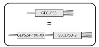
One GECLPS3-2 and one 24VDC, 100W, Class 2 Tetra LED Driver will be required to replace each GECLPS3 or up to four GECLPS4 LED drivers.
