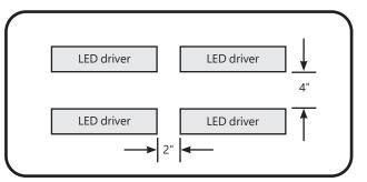
If installing multiple LED control modules or LED drivers in the same compartment, keep them at least 2" (50.8mm) apart end to end and 4" (101.6mm) apart along the sides.
