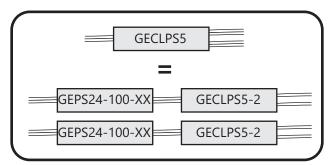
Two GECLPSPH-2 and two 24VDC, 100W, Class 2 Tetra LED Drivers will be required to replace each GECLPSPH LED driver. One GECLPSPH-2 and one 24VDC, 100W, Class 2 Tetra LED Drivers will be required to replace each GECLPSPHA LED driver.
