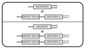
Two GECLPSPH-2 and two 24VDC, 100W, Class 2 Tetra LED Drivers will be required to replace each GECLPSPH LED driver. One GECLPSPH-2 and one 24VDC, 100W, Class 2 Tetra LED Drivers will be required to replace each GECLPSPHA LED driver.
