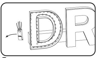
Remove the existing GECLPSPH. Do not remove existing channel letters and wiring.
