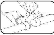
8 Plug together all adjacent Tetra Contour LS sections and tuck wires behind.
