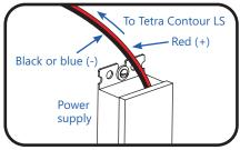
Run a wire from the power supply to a section of Tetra Contour LS.
