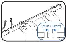
5 Continue attaching all the sections to the remaining mounting clips, leaving a 3/8 inch (10mm) gap between sections to allow for expansion or contraction.
