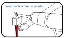
Secure the weather box using a #6 or #8 (M2 or M3) screw.
