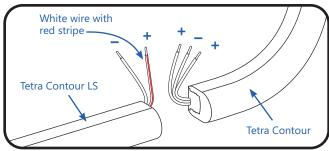
Tetra Contour LS can be connected to formable Tetra Contour for custom shapes. Separate wires and identify conductors as positive (+) and negative (-). Strip ends back 0.5 in. (13mm).
