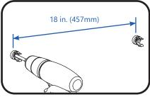
1 Install one mounting clip at each end and then a minimum of one mounting clip every 18 inches (457mm).
