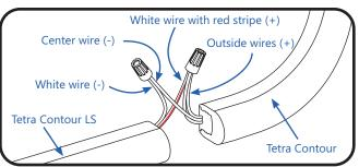
2 Splice the white wire with red stripe (+) of Tetra Contour LS to the two outside wires (+) of Tetra Contour and splice the white wire (-) of Tetra Contour LS to the center wire (-) of Tetra Contour. Insert wire connectors into weather box. Fill with electrical grade silicone and close box.
