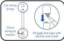
For vertical or near vertical installations, we recommend designing such that any cut-end termination of a Contour piece resides at the top of the design.
