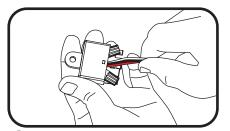
(16) Insert wire connectors into weather box. Fill with electrical grade silicone and close box.
