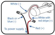
Using twist-on wire connectors, connect the white wire with red stripe (+) from the LED strip to the red wire (+) of the power supply. Connect the white wire (-) from the LED strip to the black or blue wire (-) of the power supply.
