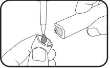
3 For cut end, fill cap with electrical grade silicone and push cap on the end to seal. Clean excess silicone.
