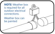
9 Insert wire connectors into weather box. Fill with electrical grade silicone and close box. Weather box can be mounted using #8 (M3) screws.
