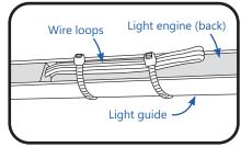
Wires between light guide segments can be folded behind the light guide and attached with clear zip ties.
