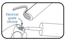
For uncut end, fold wire over Tetra Contour. Fill the end cap with silicone and push cap on the end to secure. Clean excess silicone.
