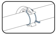
6 Secure light guide by twisting tie-wire around the mounting clip and light guide.
