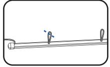
2 If required, using a sharp cutting tool, cut wire loops between sections (refer to the Cutting Resolution Table on page 2). Remove light engine from light guide and cut light guide to desired length.
