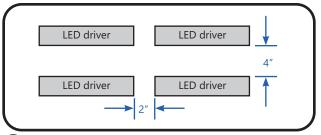
If installing multiple LED drivers, keep them at least 2" (50.8mm) apart end to end and 4" (101.6mm) apart along the sides.
