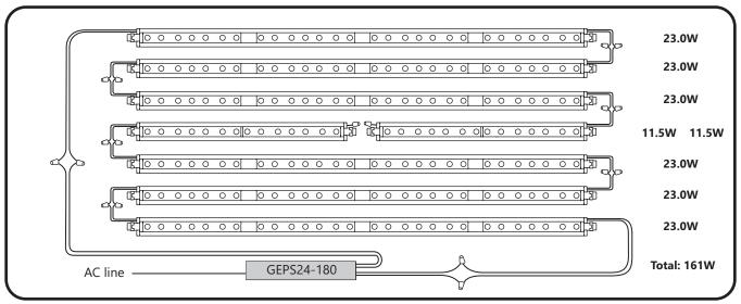
Connect Line Fit Lights using twist-on wire connectors or in-line (IDC) connectors. Join white wires together and red striped wires together. Cap all exposed wires with appropriate end caps or apply electric grade (non-corrosive) silicone for additional weather protection.
