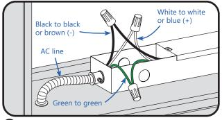
Wire AC line to LED driver(s) in accordance with the applicable local, state, and country electrical codes. Connect black to black or brown, white to white or blue, and green to green using 18 AWG (0.82mm²) wire connectors.
