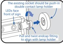
Orient Line Fit Light so LEDs are facing front of sign, then pull and twist the two endcap fittings so they align with existing fluorescent lamp holders.
