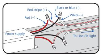
4 Connect the red stripe wire (+) of the LED system to the red wire (+) of the power supply. Connect the white wire (-) of the LED system to the black or blue wire (-) of the power supply.
