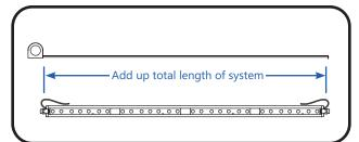
1) Add up total footage of the system to determine the appropriate number of 24VDC Class 2 LED drivers to use based on the **Power Supply Loading** chart on last page.
