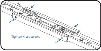
Using a screwdriver tighten all four set screws to secure the assembly. **Tighten screws until resistance is felt, then tighten additional 1/2 turn.**
