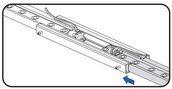
3 Slide the second LFL-LED light bar into the other end of couplers. Ensure both sides are fully inserted up to the hard stop feature.
