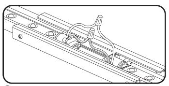
5 Connect the wires between the two LFL-LED light bars.
