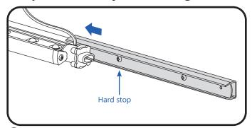
1 Match up key-slot feature on one coupler with the LFL structural rail. Slide coupler onto LFL until it hits the hard stop. Ensure power wire is folded back and away from coupler.
